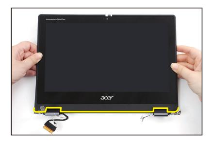
Figure 1-31. LCD Panel Removal
