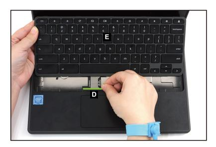
Figure 1-22. Keyboard Removal
