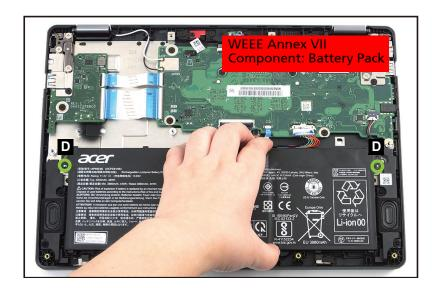
Figure 1-8. Battery Pack Removal
