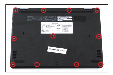
Figure 1-3. Base Cover Removal
