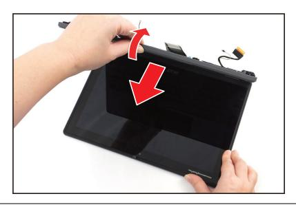
Figure 1-18. LCD Module Removal
