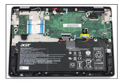
Figure 1-7. Battery Pack Removal
