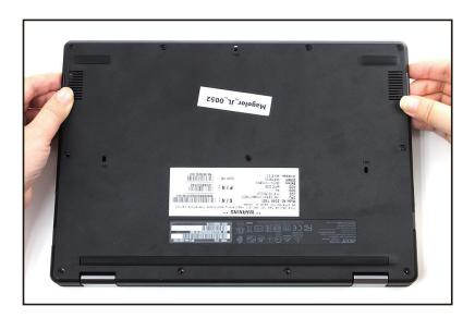
Figure 1-5. Base Cover Removal
