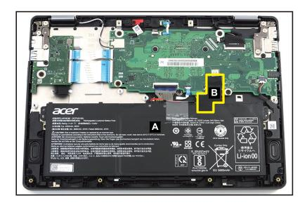
Figure 1-6. Battery Pack Removal
