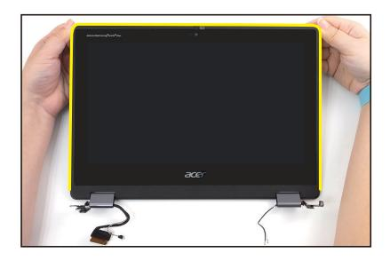
Figure 1-30. LCD Panel Removal
