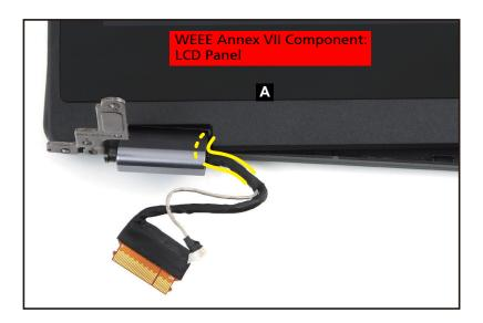
Figure 1-32. LCD Panel Removal
